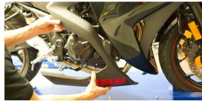
Remove OEM muffler assembly. Muffler mounting bolt will be re-used with TBR muffler.
