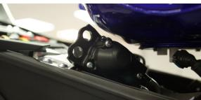
Remove the servo cap and disconnect the cables.
