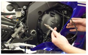
8. Before you run the bike, clean off all fingerprints and dirt, as any oily residue will etch the metal and become somewhat permanent when the system gets hot. Run the bike and enjoy. It is normal for some white smoke to appear the first time you start the bike. This is packing/manufacturing oil from inside the pipe burning off. Check for gaps or leaks. If you find a leak, a little high temperature silicon sealant should fix it. After 50 to 100 miles, recheck all fasteners for tightness.
