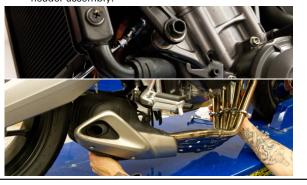
Remove plate from lower frame rail. Save hardware for use with TBR bracket.
