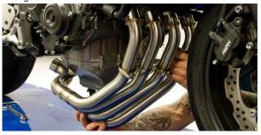
Apply anti-seize to O2 sensor threads and install onto TBR head pipe.
