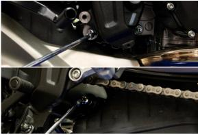
5. Remove O2 sensor from OEM muffler.
