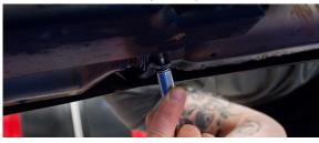
8. Remove OEM muffler mounting hardware.
