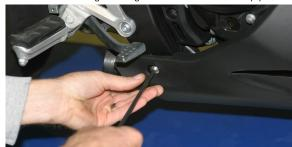
4. Remove header mounting bracket hardware, save to re-use later.
