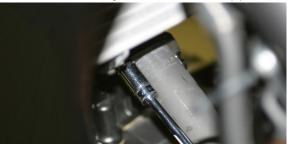
Install header pipe using OEM flange nuts and support bracket bolt with OEM hardware.
