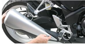
B. Remove rear right fairing mount to access header pipe bolt.
