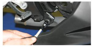
. Remove header flange nut and remove header pipe.
