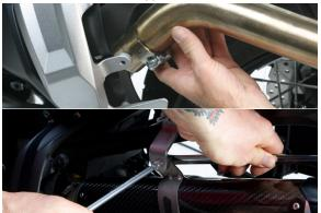
7. Make sure muffler is properly aligned, then tighten all the bolts in this order: Muffler mount bolt, muffler clamp bolt, slip-tube barrel clamp.
