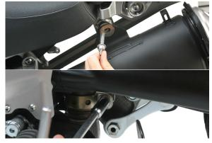
4. Install TBR muffler bracket with OEM mount bolt and nut, leave loose for now.
