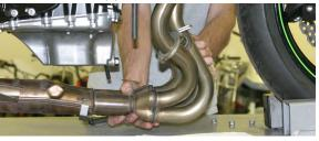
11. Using the OEM copper gasket between header collar and cylinder head. Install TBR header using OEM bolts.
