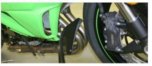
Remove header pipes.
