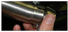
8. Install the TBR muffler assembly to the motorcycle using the supplied 8x20mm socket head flat bolt and dished washer and 8mm flange nut.
