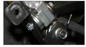
Attach the TBR slip-on tube to muffler using the 4 6x20mm socket head cap screws and 6mm split washers provided. Leave loose for now.
