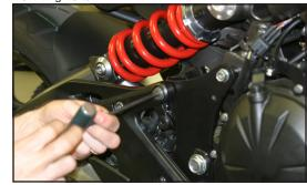
4. Remove muffler mounting hardware.
