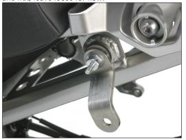
Loosely attach TBR slip-tube to TBR muffler using the supplied two-part X-Ring and 6x20mm bolts with lock washers.
