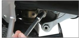
Install TBR muffler bracket with OEM mount bolt and nut, leave loose for now.
