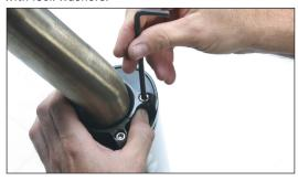
Install TBR muffler assembly to motorcycle with the rubber lined muffler clamp on muffler and barrel clamp on slip-tube. Muffler clamp attaches to outside of muffler bount bracket with supplied bolt, nut and washer.
