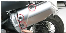
Remove OEM exhaust by removing mounting bolt and loosening mide tube bracket.
