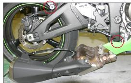
Remove lower right footpeg bolt and replace with supplied 8x35mm bolt.
