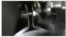
12. Check alignment of the exhaust and clearance from swingarm and and tighten the 4 6x20mm V.A.L.E.™ bolts.
