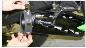
11. Loosely install muffler clamp to TBR bracket using the supplied 8x20mm bolt and nut.
