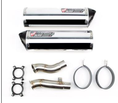
Adjust and align mufflers and tighten the X-ring bolts. Then muffler joint clamp and muffler mounting clamps last.
