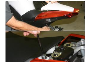
3. Remove support bracket under main seat assembly.
