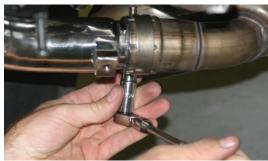
canister clamp(s). Run the bike and enjoy. It is normal for some white smoke to appear the first time you start the bike. This is packing/manufacturing oil from inside the pipe burning off. Check for gaps or leaks. If you find a leak, a little high temperature silicon sealant should fix it. After 50 to 100 miles, recheck all fasteners for tightness.
