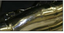
Attach muffler to TBR slip system using the supplied X-ring, 6x14mm socket head cap screws and lock washers that are provided, leave loose for
