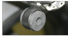
7. Re-install O2 into Slip-tube bung.
