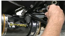
17. Check alignment and tighten muffler and the 4 6x14mm V.A.L.E.™ socket head cap screws.
