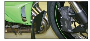
10. Remove header pipes.
