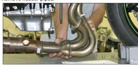
11. Using the OEM copper gasket between header collar and cylinder head. Install TBR header using OEM bolts.
