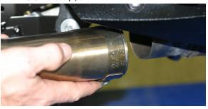
6. Carefully slide the canister clamps over each of the canisters. Make sure the TBR muffler canister sits straight. (Note: The stainless steel canister clamp and the name badge on the canister come from the factory with a clear plastic protective film. Please remove this film before operation).
