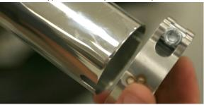
Insert the slip tube of each V.A.L.E.™ muffler assembly into OEM head pipe.
