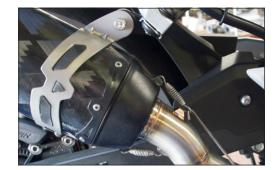
Install center stand rubber bumper (use the OEM rubber bumper and install it onto the TBR slip-tube bracket).
