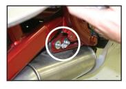
5. Remove the two muffler mounting bolts and remove the OEM muffler. You will re-use the front muffler mount bolt and the rear flange nut.
