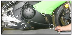
3. Remove the four fasteners on the right side cover.
