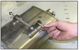
6. Remove the rubber grommet and inserts from the frame where the stock muffler mounted on the left side.
