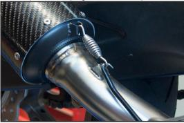
10. Make all adjustments of slip-on tube rotation and muffler rotation to make sure there is clearance between swingarm/tire and brake pedal when applied.
