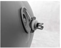
3. Use any high pressure pump with a Halkey-Roberts valve adapter to inflate to desired firmness. Insert the pump hose adapter into the valve and twist **clockwise** ¼ turn to secure. The valve will automatically open when the hose is inserted correctly. Do not exceed 10psi.
