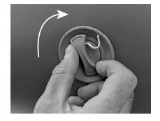
6. Replace valve cap by inserting into valve and twisting **clockwise**.
