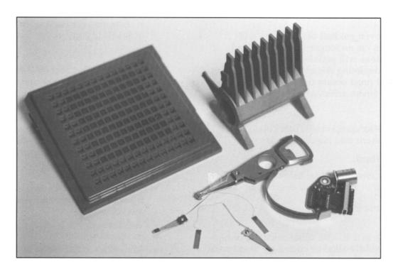
The challenge for many companies that manufacture read-write devices for computers is to eliminate the use of ozone-depleting chemicals but still obtain comparable cleanliness levels of their disk drive components. A high degree of cleanliness is critical to long-term performance and reliability of disk drive components. The demand for high storage capacity in a reduced-size disk drive makes the cleaning process increasingly important.
