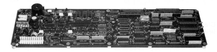
Semi-aqueous and saponified aqueous solutions offer effective alternatives to cleaning printed circuit boards whether the boards are fabricated with through-hole or surface mount devices or are mixed technology. Use of ultrasonic or MicroCoustic energy in the cleaning and rinsing process make these solutions efficient alternatives to CFC-based solvents.
