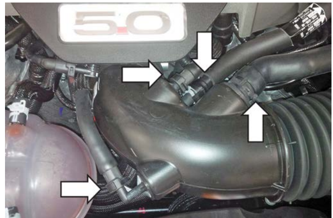
11. Using a 10 mm wrench or deep-well socket, remove the nut retaining the induction resonance tube to the firewall behind the driver side cylinder head.
