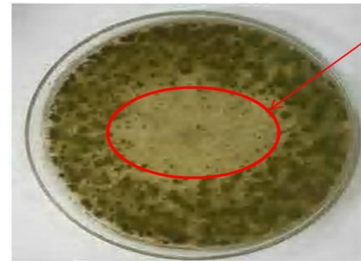
inhibition zone with 20ppm ozone /5 min
