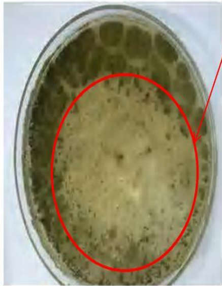
inhibition zone with 40ppm ozone /20 min
