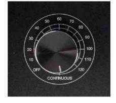
If you wish the machine to operate continuously, turn the handle anticlockwise to the position marked CONTINUOUS. Natural Ozone do not recommend the continuous use of ozone.
