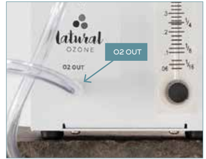
STEP 3: Using the leurl lock connector to connect oxygen tubing from O2 OUT port of Low Flow Meter to oxygen inlet on the back of the Ozone Generator. Use package C.
