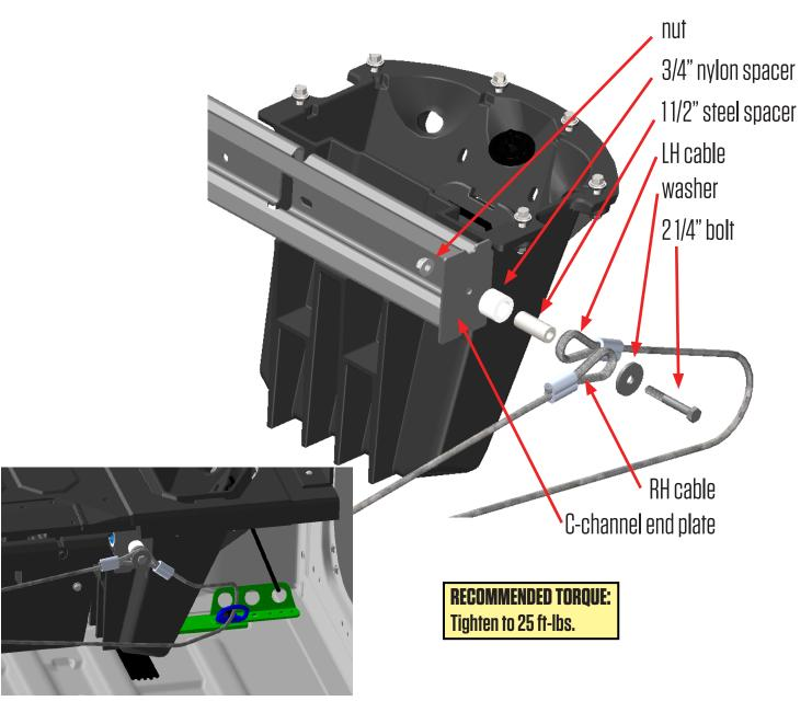
Enlargement of LH cable assembly attachment to cargo tie down loop (shown in blue). Do not loop through mounting bracket (shown in green).
