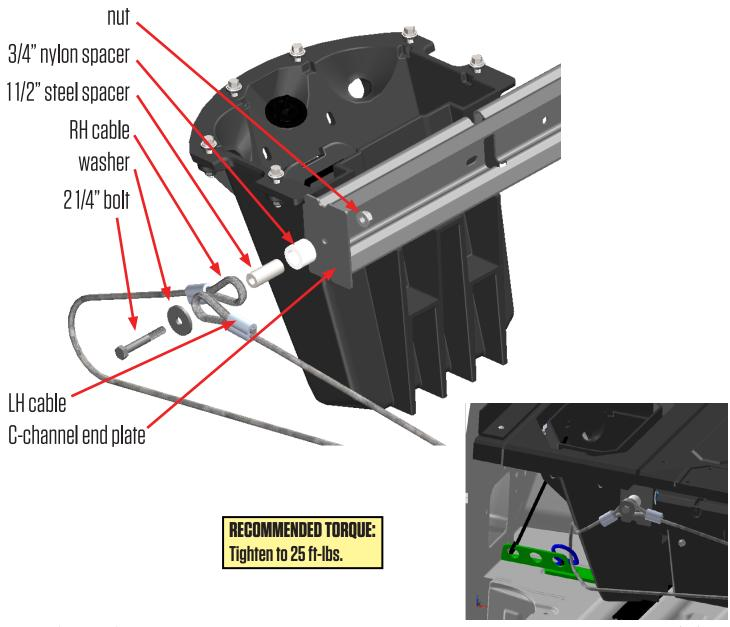
Enlargement of RH cable assembly attachment to cargo tie down loop (shown in blue). Do not loop through mounting bracket (shown in green).
