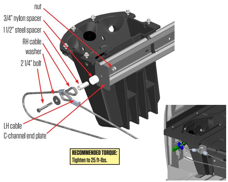
Enlargement of RH cable assembly attachment to connecting link (blue).
