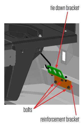
LH side reinforcement bracket shown
