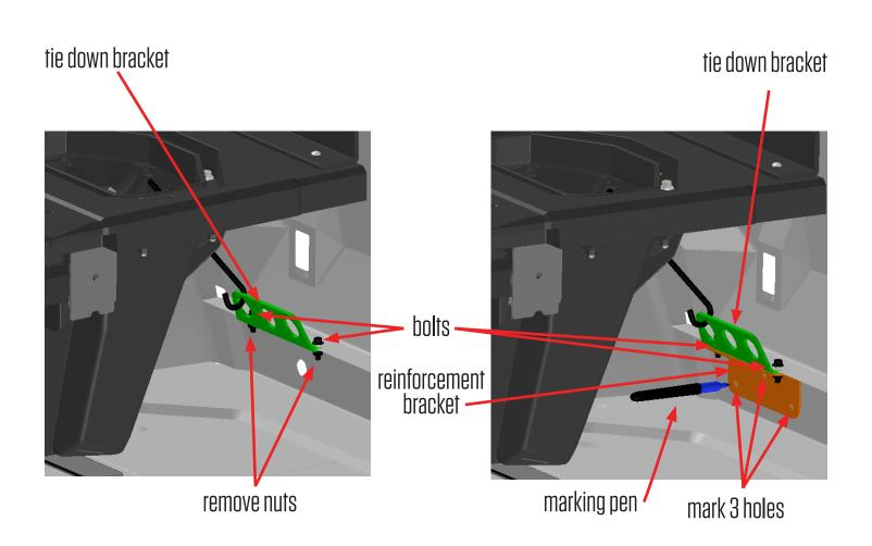
LH side reinforcement bracket shown
