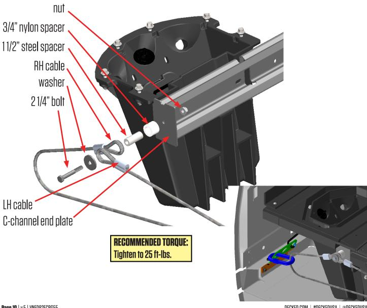
Enlargement of RH cable assembly attachment to connecting link (shown in blue).
