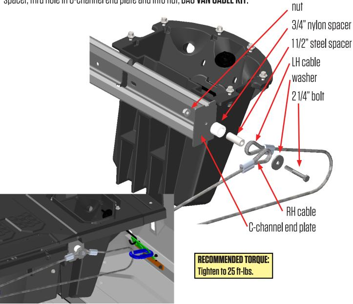
Enlargement of LH cable assembly attachment to connecting link (blue).
