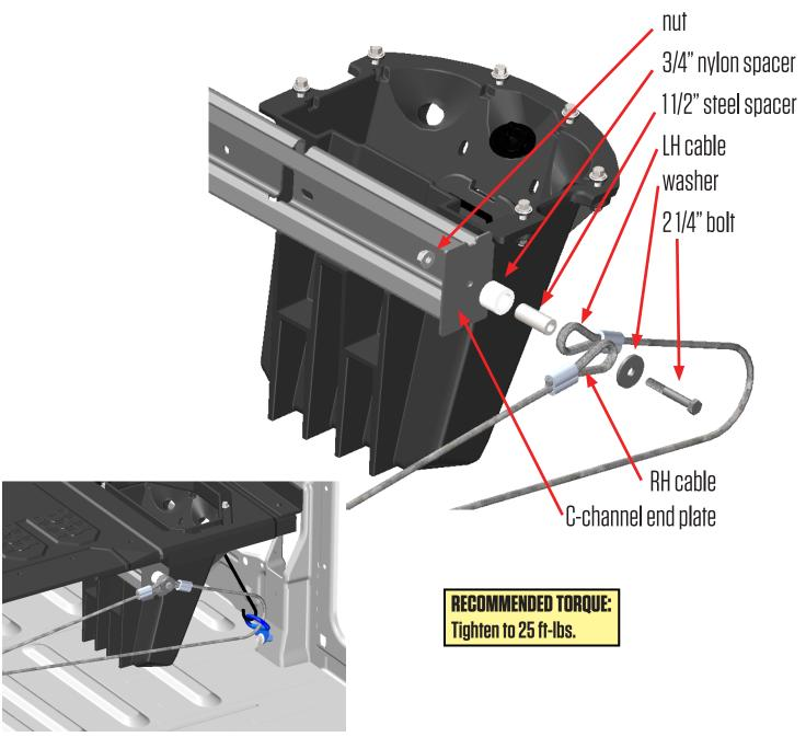
Enlargement of LH cable assembly attachment to cargo tie down loop.
