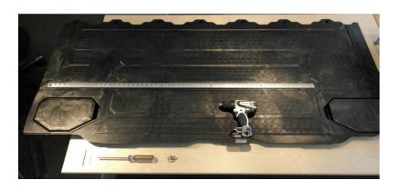
EASY MISTAKE # 2: Drill through both sides of steel tubes. <u>ONLY</u> drill through the top of steel tube.
