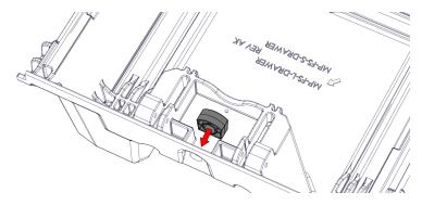
**STEP 2:** Install one rubber o-ring onto each lock barrel:
