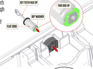
**STEP 4:** Install lock core nut and tighten with a 7/8" socket or wrench.
