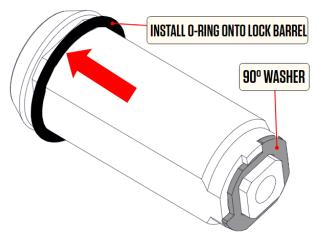
**STEP 3:** Insert key into lock core with the teeth facing up. Insert the lock core through the drawer and the anti-rotation support - note the correct position of the  $90^{\circ}$  washer.
