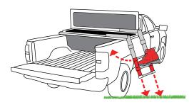
PLACE LADDER ON SOLID GROUND WITH BOTH RUNGS LOCKED INTO PLACE (LADDER STEPS 1-3). FAILURE TO DO THIS COULD ALLOW LADDER TO SWING INTO TRUCK AND CAUSE DAMAGE TO THE VEHICLE
