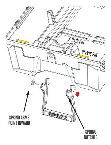
HELPFUL TIP: MAKE SURE SPRINGS HAVE THE LONG ARM HORIZONTAL AND SHORT LEG VERTICAL BEFORE INSERTING HANDLE
