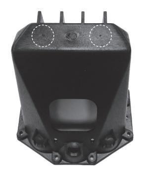
There are two dimples in the bottom of each ammo can. Drill a 1/4" hole at each dimple
