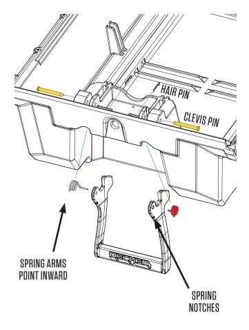
HELPFUL TIP: MAKE SURE SPRINGS HAVE THE LONG ARM HORIZONTAL AND SHORT LEG VERTICAL REFORE INSERTING HANDLE
