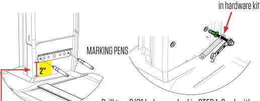
Drill two 3/8" holes marked in STEP 1. Seal with self-etching primer. Insert plusnut (green) into hole. Install 1" placement bolt through install wrench and into plusnut. While holding with installer wrench, tighten bolt head until plusnut is fully crimped. Unthread placement bolt and use again. **BAG PREP EXSV 55/65**.
