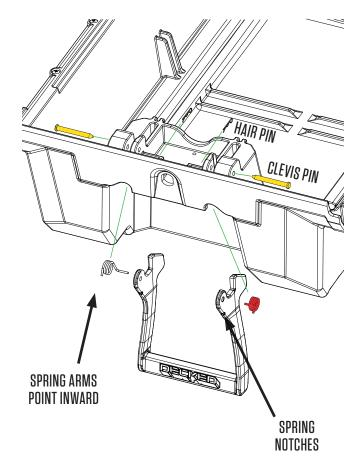
HELPFUL TIP: MAKE SURE SPRINGS HAVE THE LONG ARM HORIZONTAL AND SHORT LEG VERTICAL REFORE INSERTING HANDLE
