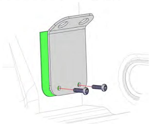
**DETAIL B:** Install DECKED cabside bracket
