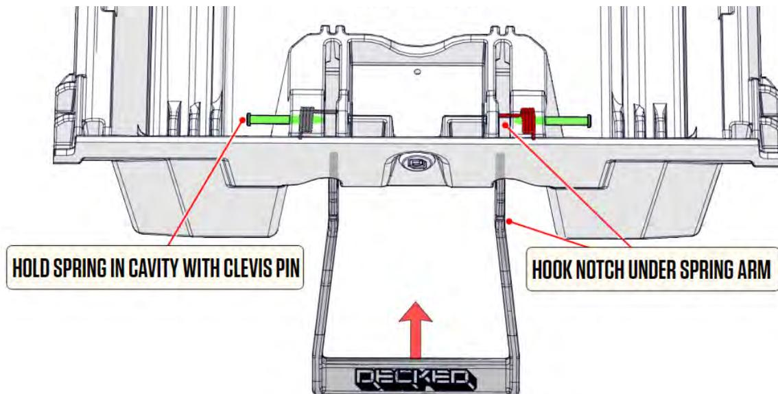
3. Install a clevis pin through each outside drawer hole and through the spring to hold the spring in place. Do not push through 2nd hole.
