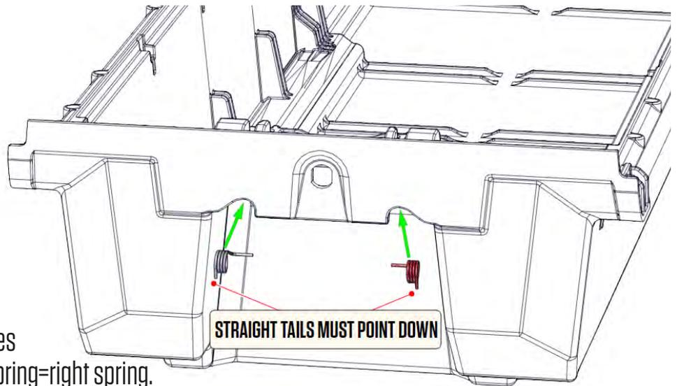
**NOTE: Each spring arm should point inward, with the straight tails facing you and pointing down.**
