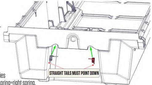
NOTE: Each spring arm should point inward, with the straight tails facing you and pointing down.
