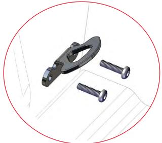
**DETAIL A:** Remove factory cabside tie down bracket
