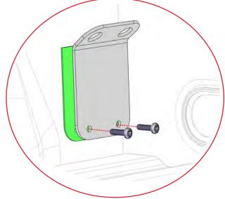
**DETAIL B:** Install DECKED cabside bracket
