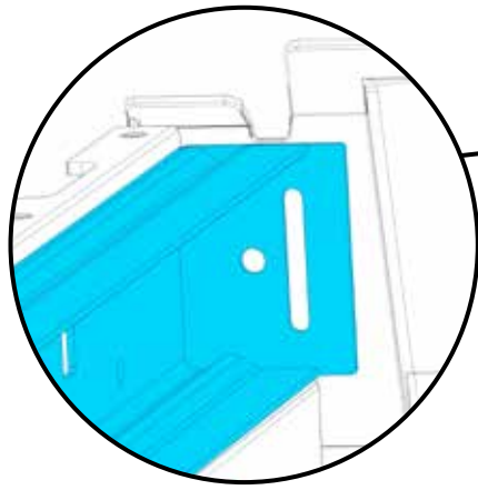
END PLATE ON CABSIDE
