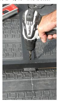
Attach the cross brace tailgate end to deck with 2" x 5/16" #18 bolts.
