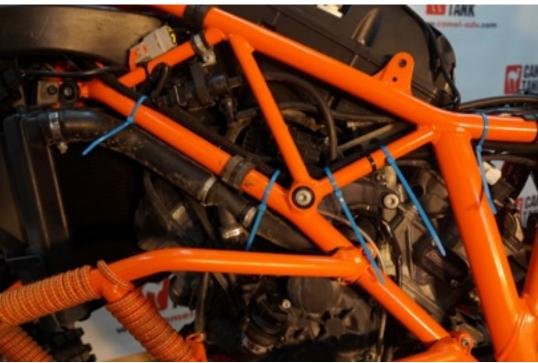
• Route fuel line under left side air intake duct and under diagonal frame support, then cross over to the right side. The hose should come out under the right side diagonal support but over the front brake hose hard lines.
