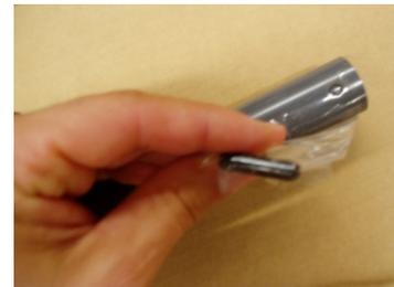
Slide the fitting off the pipe and insert the pre-drilled end into the pipe from which the fitting was removed. Ensure open end of the fittings are face down on both sides.
