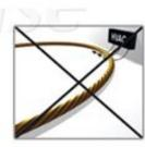
Face to air-con outlet (False alarm due to humidity)
