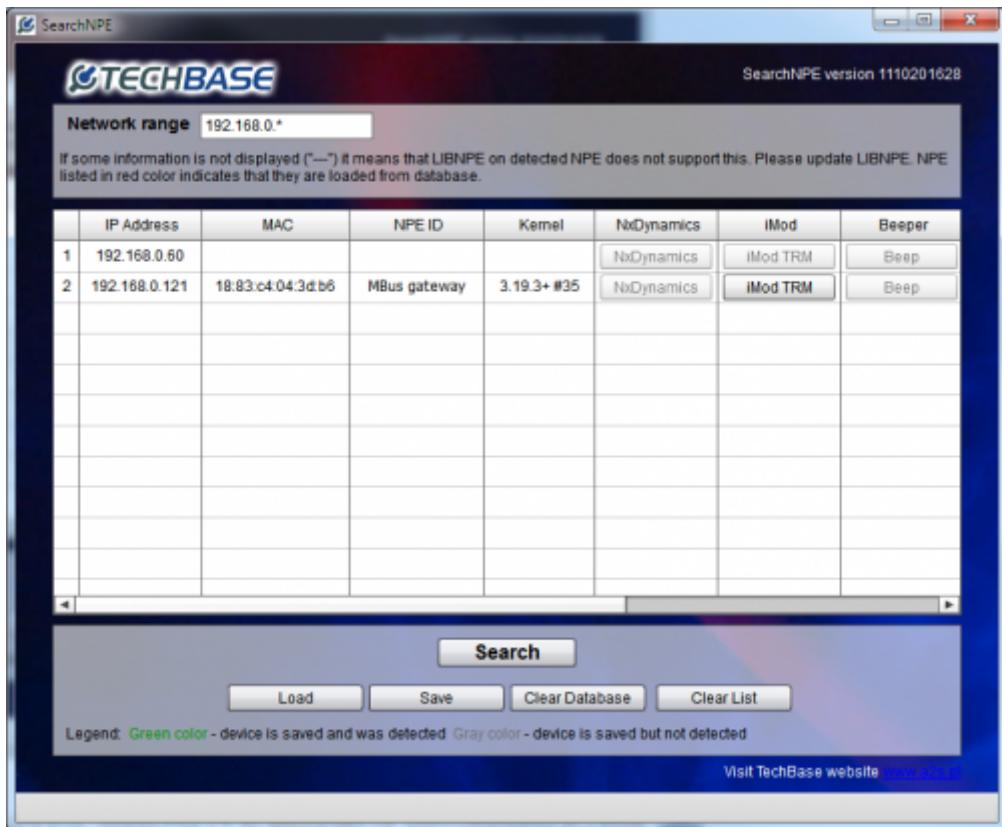
If you know IP address of the device, you can connect by SSH terminal, eg Putty. You can find PuTTY at following address: <http://the.earth.li/~sgtatham/putty/latest/x86/putty.exe>
