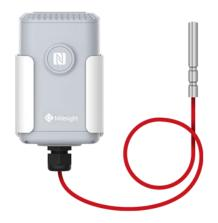
EM500-PT100 resistance temperature sensor is designed for measuring wide range of temperature in harsh environments and transmitting data using LoRaWAN<sup>®</sup> technology. With this low power consumption technology, EM500-PT100 can work up to 10 years with 19000 mAh battery. Combining with Milesight LoRaWAN<sup>®</sup> gateway and Milesight IoT Cloud solution, users can manage all sensor data remotely and visually.
