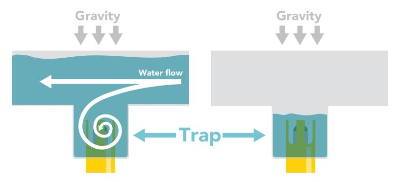
Water will collect in a trap. This water will move much slower than the rest of the water in the pipe. Your readings will seem to move slowly or become stuck. It will appear that the readings are flow rate depended (which they are not) because increasing the flow can get the readings to normalize. It reality, increasing the flow rate is simply clearing out the water stuck in the trap faster.
