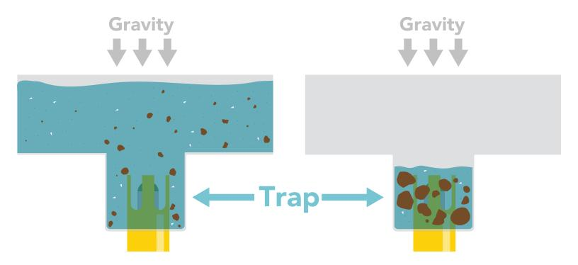
It is with 100% certainty that debris will collect in the trap. Depending on what the probe is used for that debris could be undissolved chemicals, sand, mud; you name it. Whatever it is, it is guaranteed to affect your readings.
