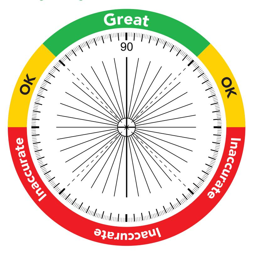
This illustration shows what angles work best when mounting a probe inline.
