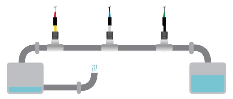
In an open system the probes can dry out. You will need to engineer a solution to this problem.
