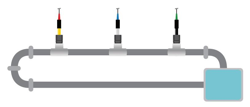
In a closed system the probes will never have an opportunity to dry out. The humidity in the pipes will be around 100% even if no water is flowing.
