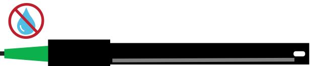
Make sure that the probe is dry before issuing this command, ec:cal,dry
