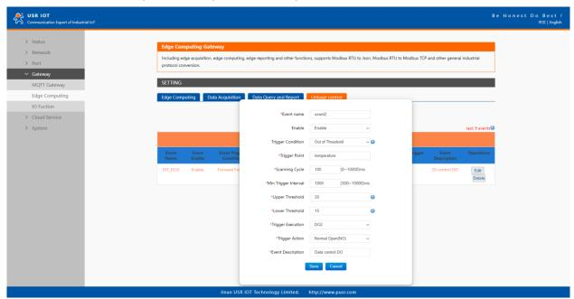
Fig. 203 Serial device data control DO
