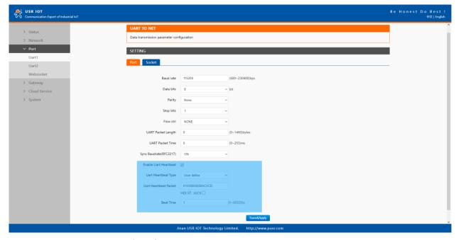
Fig. 85 Serial heartbeat packet as modbus command
