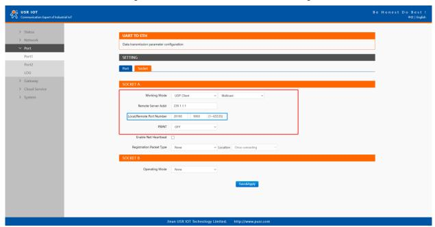
Fig. 47 USR-M100 #2 UDP multicast setting
