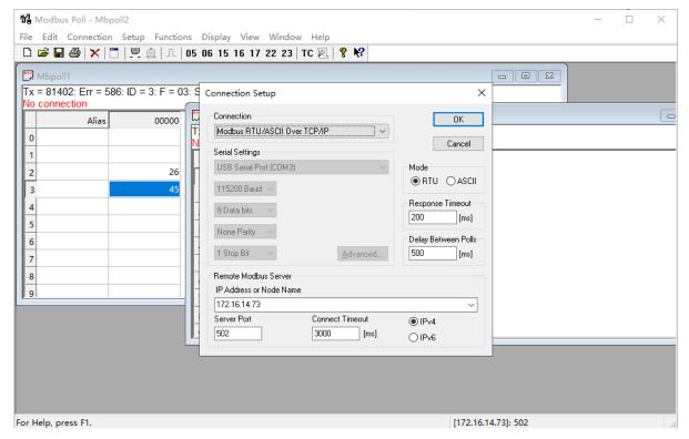
Fig. 159 Modbus RTU simulator settings
