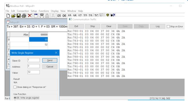
Fig. 161 Modbus RTU control and response
