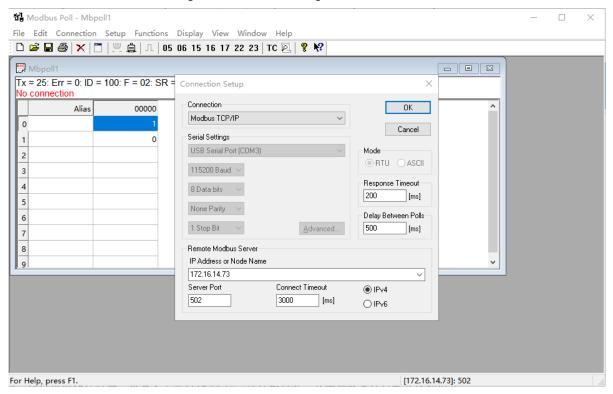
Fig. 169 Modbus TCP simulator settings
