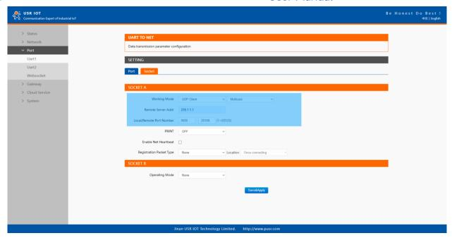
Fig. 46 USR-M100 #1 UDP multicast setting
