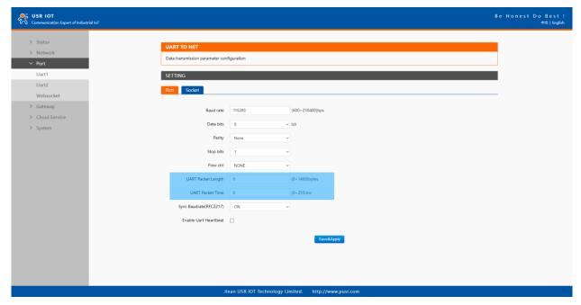
Fig. 87 Data packing mechanism
