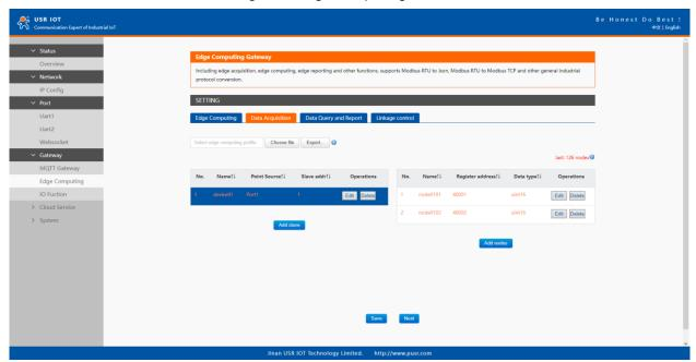
Fig. 26 Modbus slaves and datapoints configuration
