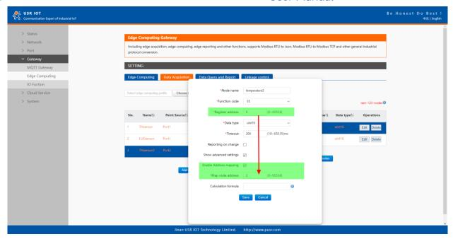
Fig. 152 Register address mapping
