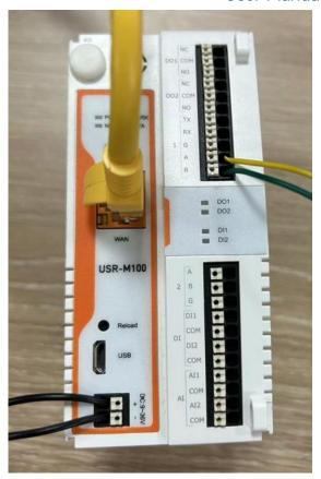
Fig. 10 Hardware connection
