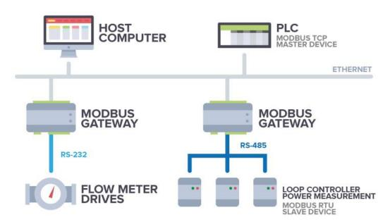
Fig. 69 Ethernet masters with multiple serial slaves
