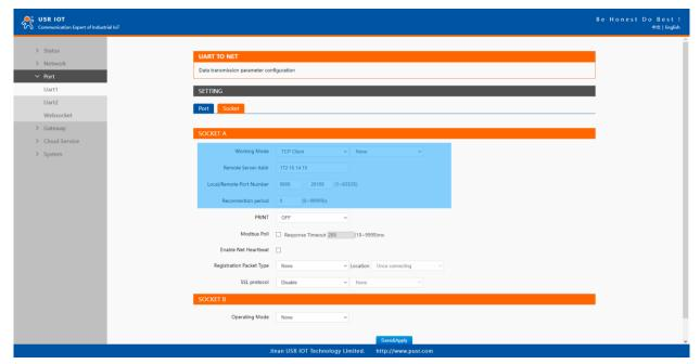
Fig. 62 TCP client mode in USR-M100
