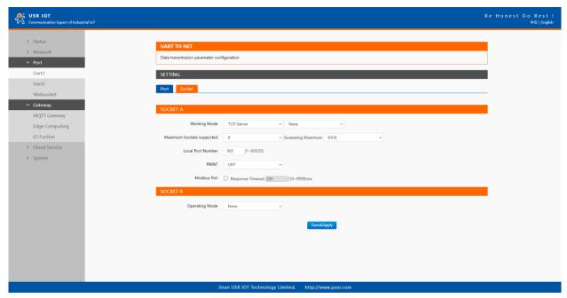
Fig. 168 Socket setting for modbus TCP
