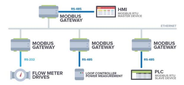
Fig. 75 Serial master with multiple serial slaves
