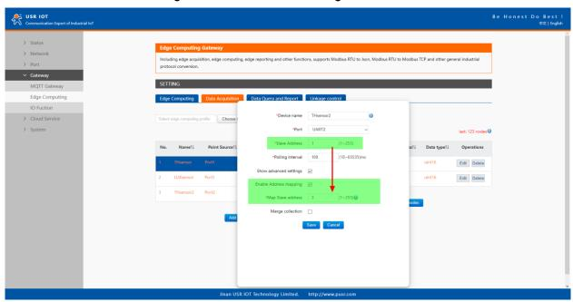
Fig. 151 Slave address mapping
