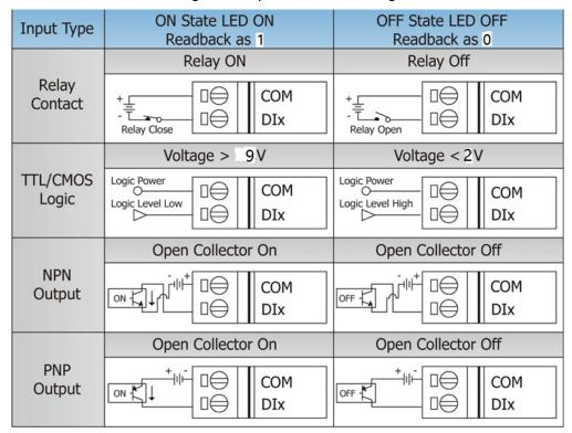
Fig. 4 DI wire connection
