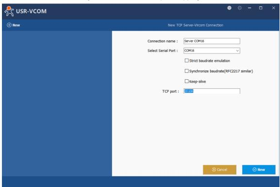
Fig. 80 Mapping a virtual COM port
