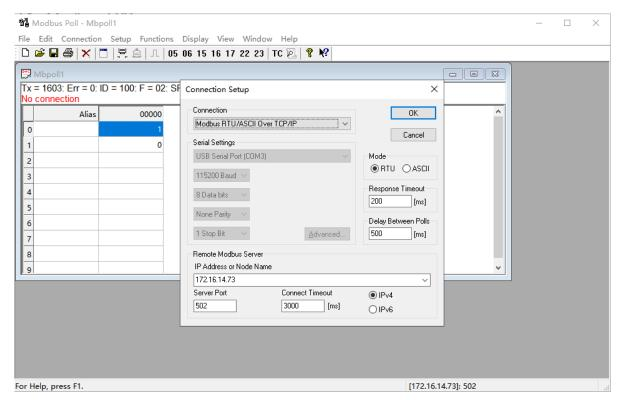
Fig. 179 Modbus RTU simulator settings
