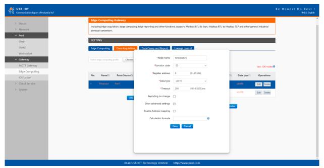
Fig. 130 Data point configuration
