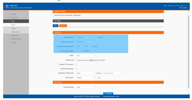
Fig. 73 Modbus TCP slave settings
