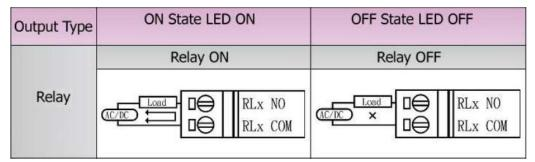
Fig. 5 DO wire connection
