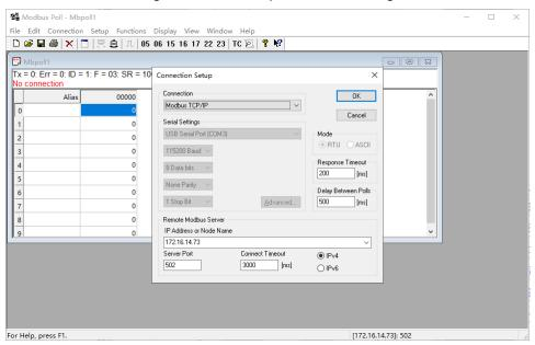
Fig. 155 Modbus TCP simulator settings
