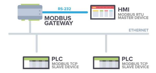
Fig. 72 Serial master with one Ethernet slave
