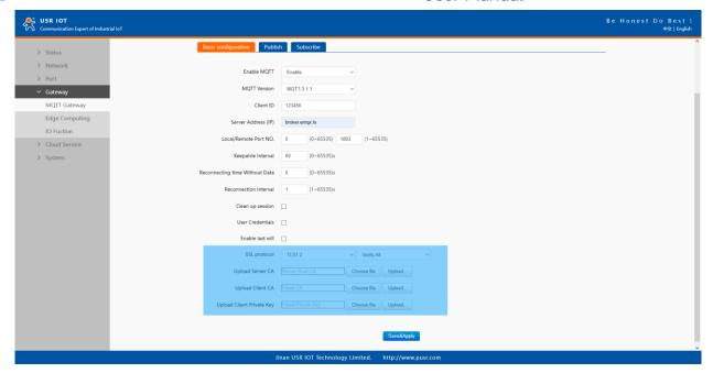
Fig. 104 SSL/TLS connection
