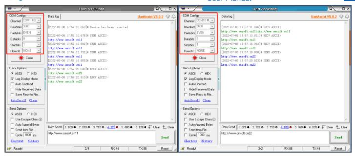
Fig. 68 Synchronizing serial port parameters
